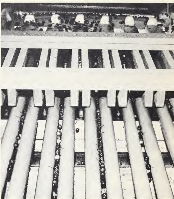
Top left: At most packing houses, cherries are dumped on conveyors and hand-sorted for defects and off-grade fruit. Top right: Stem cutters (rotating circular saws) divide clusters of cherries into individual fruit (with stems attached) to facilitate sizing. Bottom left: A water spray (often containing fungicide) is used to reduce friction during sizing, thus lessening incidence of injury. Bottom right: Diverging-roll sizer commonly used for sizing cherries.
